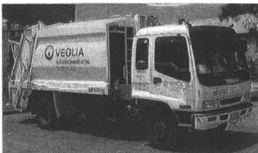
REARLIFT TRUCK 4X2 MID RANGE 10m³ & 12m³ BODY
